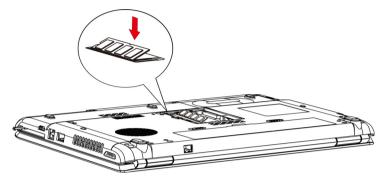
Figure 8-6 Inserting the memory module
